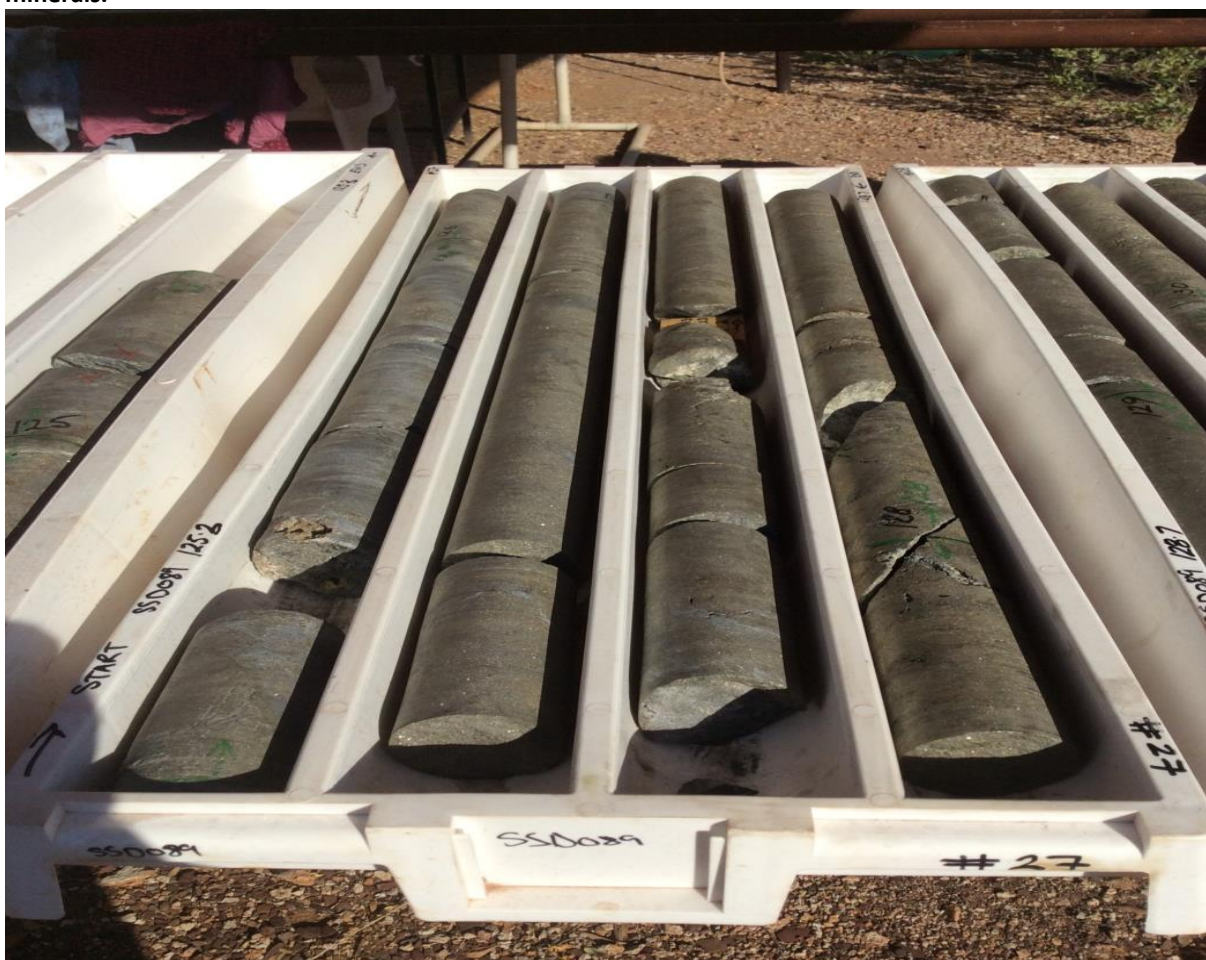
Image 2: Photograph of indicative massive sulphides intersected in SSD089. Photo shows 125.2-128.7m down-hole.
