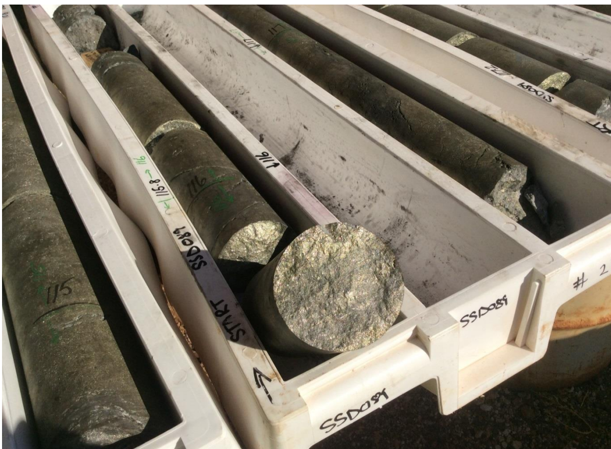
Image 1: End section of PQ core at approximately 115.8m down-hole showing visible copper sulphide minerals.
