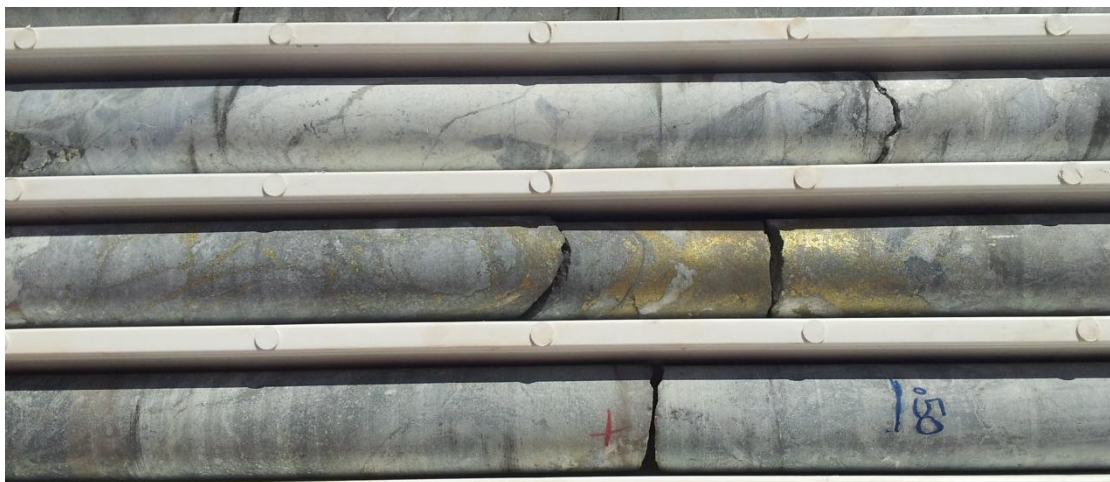
Figure 3: Stringer chalcopyrite intersected in BLD004 at the Bledisloe target area
